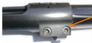
a. Barrel clamping bolts
