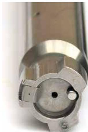
The recessed face bolt head locks directly into the breech of the barrel. The three lugs give the bolt handle a lift of 60 degrees. The S stamped on one locking lug indicates the bolt is suitable for standard calibres. The slot in the bottom left locking lug is used to locate the barrel in the receiver.
