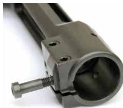
The split receiver ring. The dual screws on the side are tightened to secure the barrel in place. The front action screw goes into the recoil lug, which is integral with the reinforcing boss under the receiver ring.
