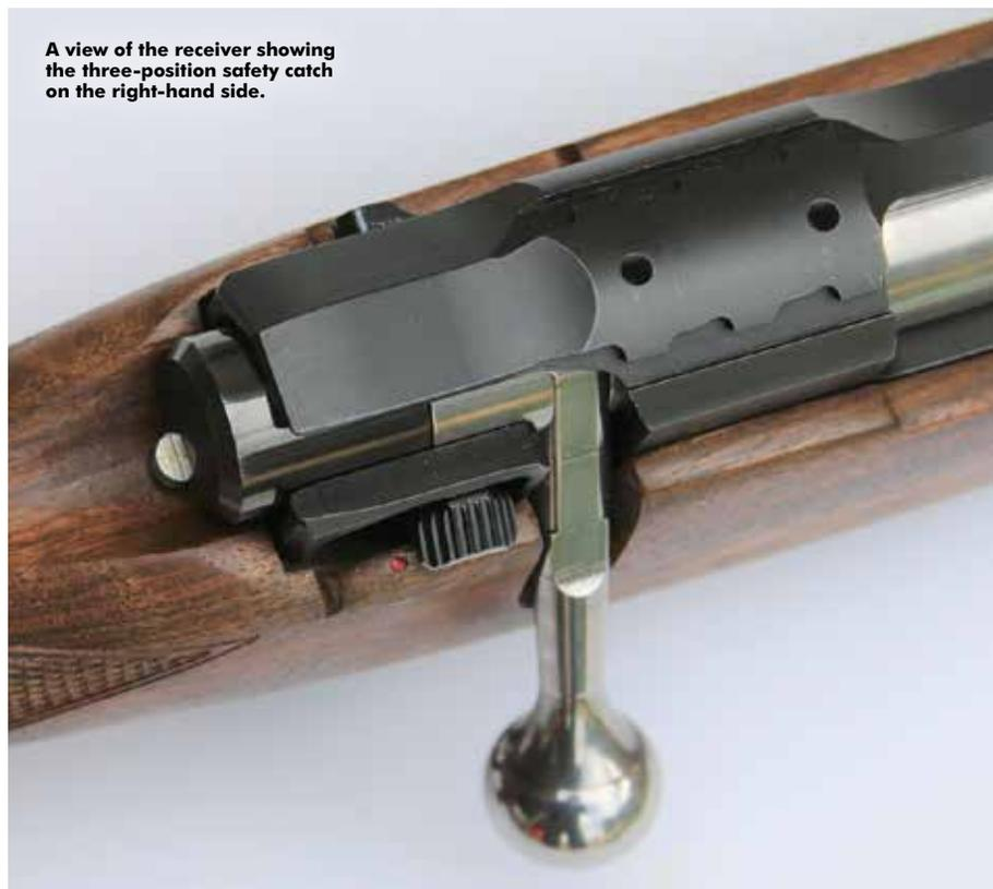
A view of the receiver showing the three-position safety catch on the right-hand side.
